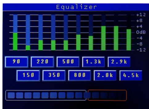
ESSB for Electret Mic. Comp level 10-20dB. EQ setup may vary differ depending on voice and microphone type
