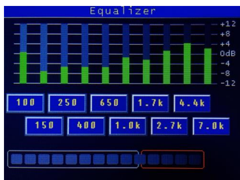
Ext CB for Electret Mic. Comp level 10-20dB. EQ setup may vary differ depending on voice and microphone type
