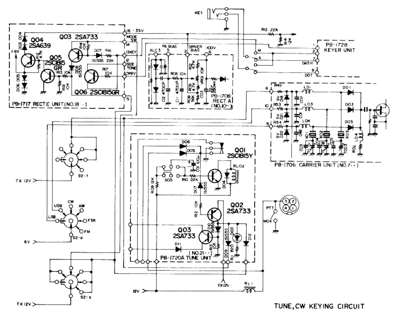
When  $D_{2107}$  is grounded,  $D_{2102}$  (2SA733) turns ON, and the voltage appearing at the collector of  $Q_{2102}$  is fed through  $D_{2109}$  (1S1555) to  $D_{701}$  on PB-1706 to activate the CW carrier oscillator. In the SSB mode, the SSB carrier oscillator is disabled by reverse voltage.
