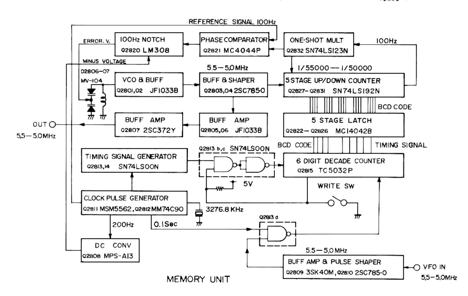
is amplified by  $Q_{2805}$  and  $Q_{2806}$  (both JF-1033B) and  $Q_{2807}$  (2SC372Y), and fed through a diode switch to the PLL UNIT (replacing the VFO signal).
